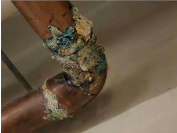
**Photo #99** Close-up of excessive electrolysis corrosion that may lead to leaking pipe soon.
