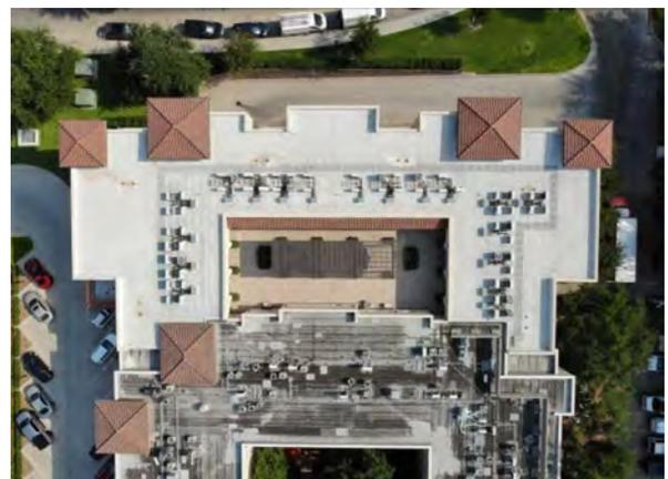
**Photo #30** Overview of modified bitumen roof over the Plaza North Expansion.
